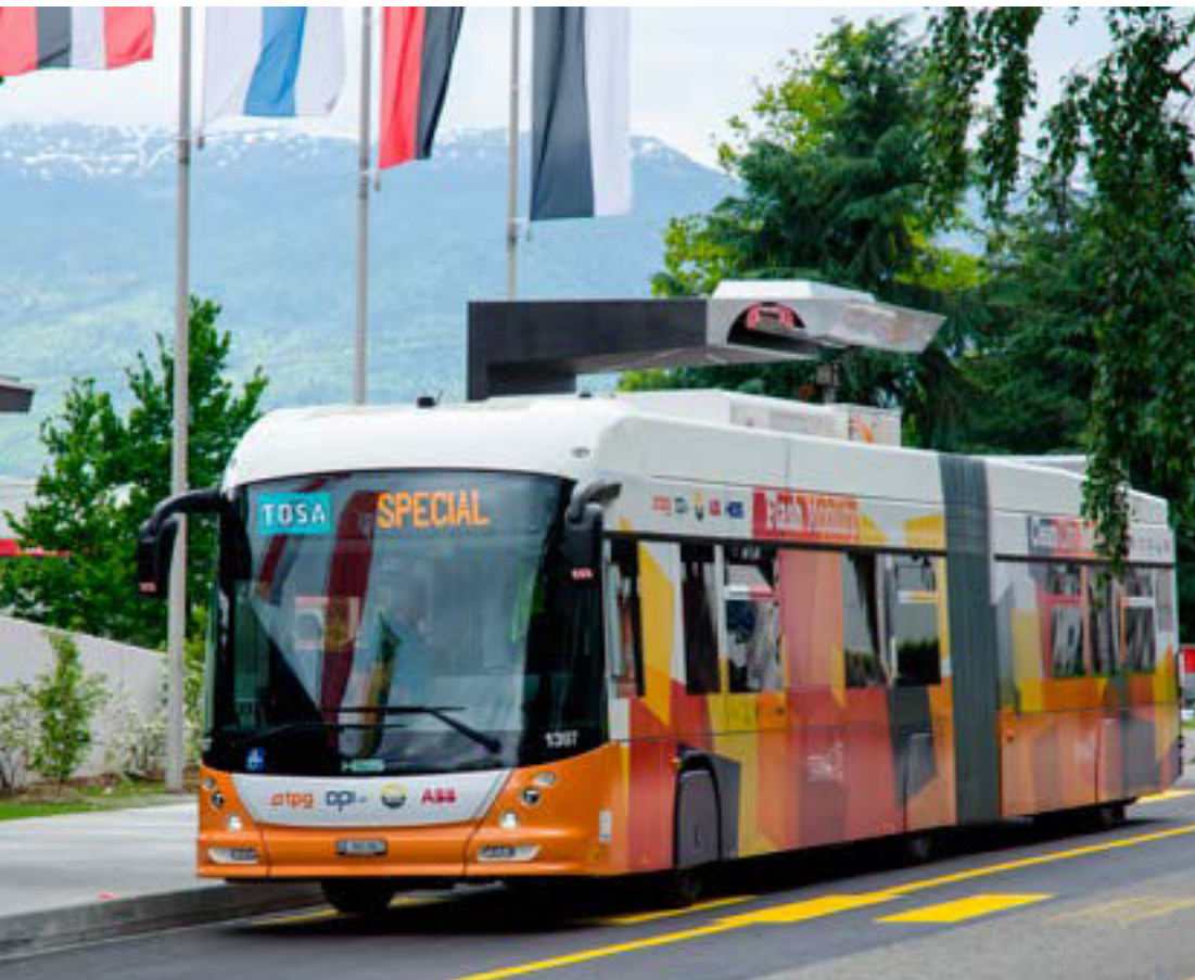
TOSA Bus, developed by ABB: No overhead lines and ultrafast charging times at bus stops pave the way for the next generation of silent, flexible, zero-emissions urban mass transit.
